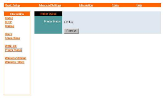
The Printer Status panel shows whether a connection to a printer can be detected on the Wireless Gateway's printer port. If the connection to the printer is good and the printer is on, printer status will be given as "On line"; otherwise it will be given as "Off line."
